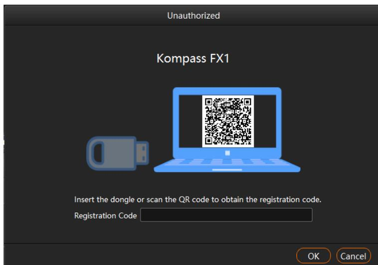
When the dongle is inserted and recognized normally, the above window and the **Kompass FX1** text on the output will disappear automatically.
